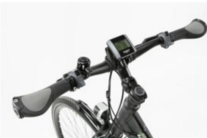
**LEFT** Superb: *Shimano* is the first supplier to bring to market both gearing and power assist systems controlled by a single consistent, unified set of user controls. The selected gear and power assist level are shown on the display at the centre of the handlebars.
