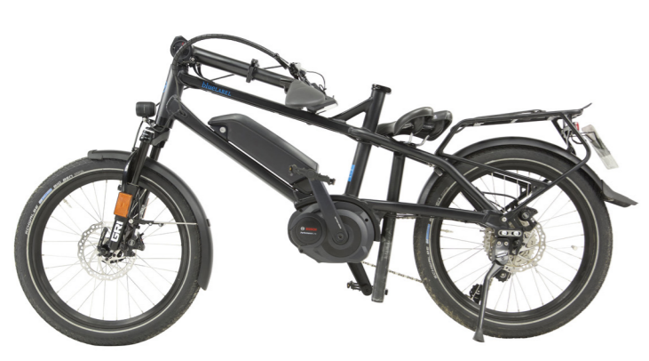
LEFT The blueLabel Pony is a pedelec 45, hence legally no longer a bicycle, so it cannot be carried with you onto a train. Thanks to the folding system in the steerer tube it can be made very flat without tools, a very practical feature for fitting it into a car or mobile home. The folding mechanism also makes it possible to make major adjustments to the riding position, from upright to sportily leaned-over.
