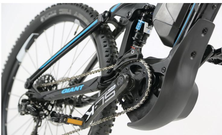
**LEFT** The Yamaha bottom bracket motor is very well integrated on this *Giant* off-road pedelec. The *Full-E+ 0* is one of the few bikes without any Shimano components. Brakes, crankset, gears and shock all come from SRAM and prove that it's perfectly possible to build a very good pedelec without Shimano components. A push assist mode and a self-explanatory on switch are top of the wish list.
