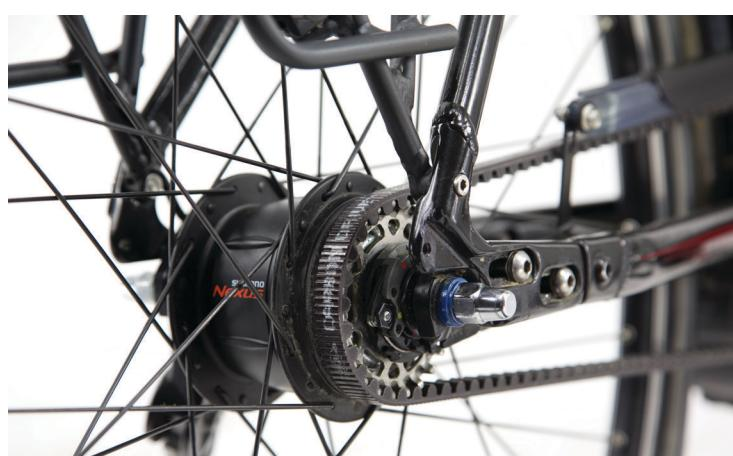
LEFT A unique combination of Gates belt drive, Shimano hub gears and Impulse mid motor with shift sensor, which throttles back the motor power during the shift process so that the shift lock in the hub gear disengages, and so that the shift is as a rule completed promptly. The price for this easy shifting is that you lose a little momentum.
