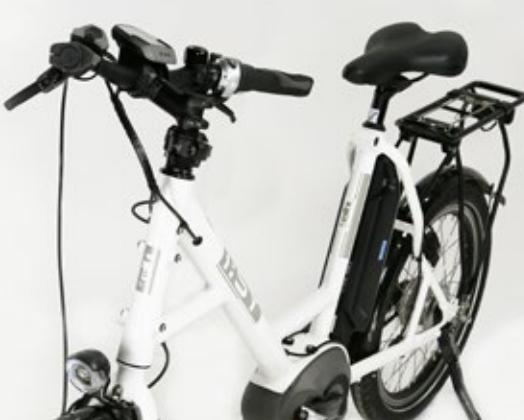
**LEFT** The *I:SY* only reveals its true size once you've used the tool-free Speedlifter stem to turn the bars through 90 degrees, and folded the folding pedals. This makes this pedelec into a very thin, low package, so that it can be easily stowed away, for example in a mobile home or car. This ability could also be just as much of an advantage in a cramped garage, or when taking it with you on public transport.
