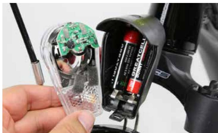
**LEFT** Legal, but potentially unpractical for everyday use: the lights are not powered from the main drive battery, but instead, to save wiring, by small batteries in the lights themselves. It's clear that the first time you'll notice the batteries are flat is when you're out and about in the dark. Also, the front and rear lights each need to be switched on and off separately.
