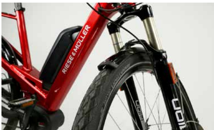
LEFT Full fat: the Schwalbe Marathon Deluxe tyres are a hybrid of the well-proven Marathon model and the comfortable shock-absorbing Big Apple tyres. The Suntour Aion suspension fork has plenty of travel too, and it is equipped with a through-axle system and the orange side reflectors which are mandatory in Germany for pedelecs 45.
